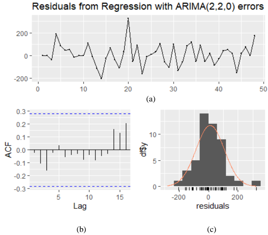
Figure 4.12: Ljung-Box Test Results of Estimated Model for Model 2: (a) Residuals Plot from Week 1 to 48, (b) Autocorrelation Function of Residuals, and (c) Histogram of the Residuals
