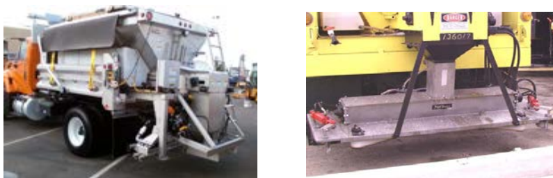
Figure 2: An on-board pre-wetting system (right) and Zero Velocity Dispensing Unit (left);.
